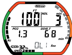
Figure 20. Oxygen Limit (OLI) Warning (grey segments flash)
