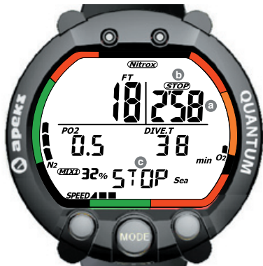
Figure 16. Safety Stop Display
